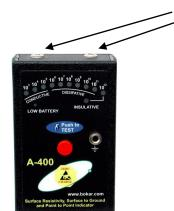
Jacks to connect the wires for point to point resistance check (Wires are supplied with the unit)
